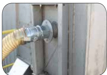
Dedusting nozzle on head section
