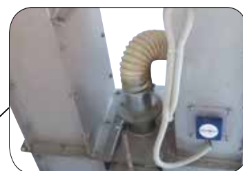
Dedusting nozzle on foot section
